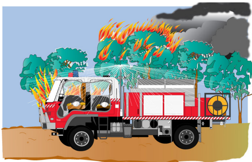
Crew are being showing visible under their blankets for diagram to show positions only. They will normally be fully covered with no part visible.
